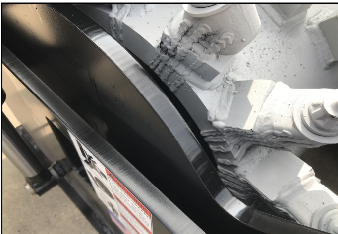
1.5 inch cutting drum with hardfacing
