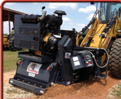
RH4075 stabilization on tool carrier
