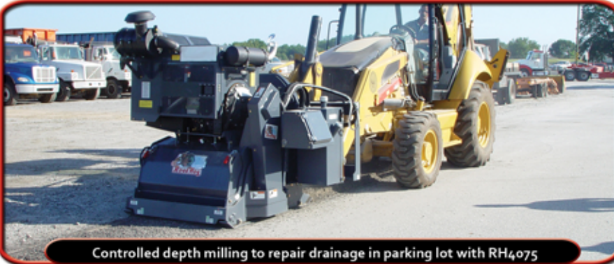
Controlled depth milling with RH4075
