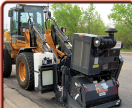
Controlled depth milling with RH4075
